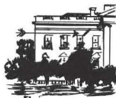
The second, "Crack Over Window", is a straight line crack running upwards and slantwards from the third window in from the left, from the lintel to the frieze. It is positioned at R18/2 on sheet 1A.
